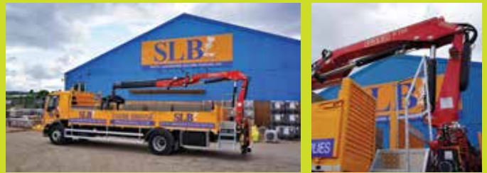
18T GVW WITH REAR AND FRONT MOUNTED FASSI F110B.1.22
