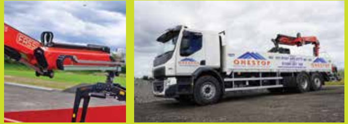
26T GVW WITH REAR MOUNTED FASSI F155A.2.22
